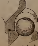
Fig. 13. Enlarged Section showing India-rubber Ball.
